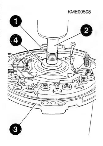
DISMANTLING AND CHECKING ALTERNATOR Dismantling pole body Slacker off bolt (1) of pole body. Detach connection/terminal B+ (2). TORX T25: comm. avail.
